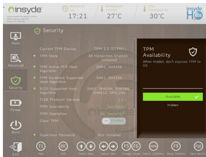
Figure 13 - Make TPM Visible
