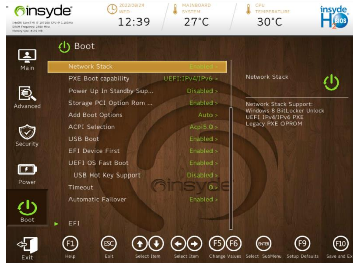
Figure 9 - Network Stack Control
